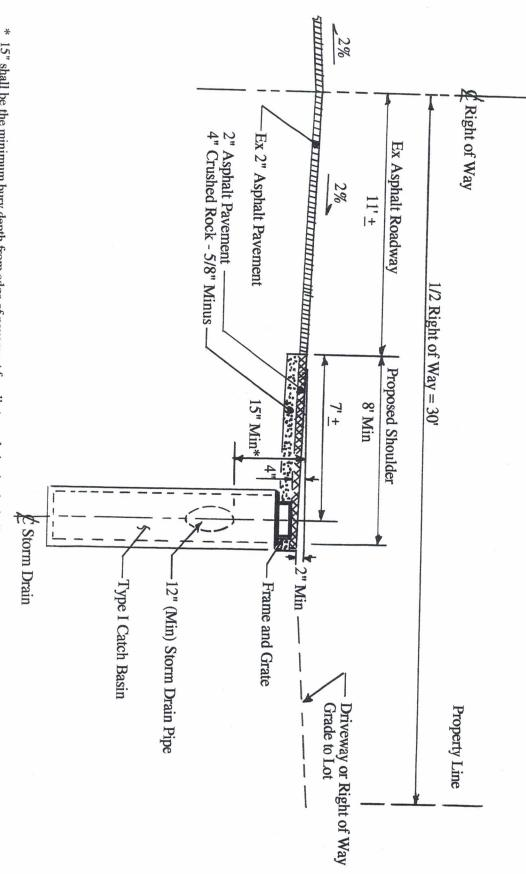
\* 15" shall be the minimum bury depth from edge of pavement for all storm drain pipe including culverts at driveways in the absence of any engineered information giving detailed grades and elevations of pipe and structures. Engineered information shall always take precedence over the 15" minimum standard.
